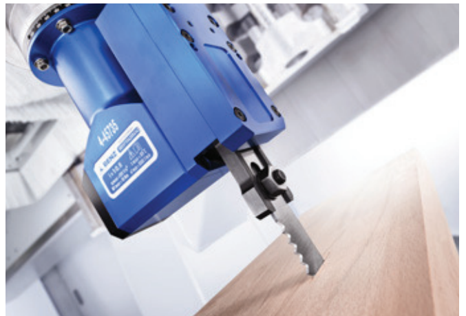
Vertical insertion of slots for fiche hinges
