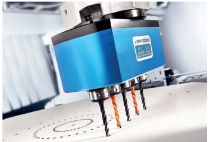
Drill rows in acoustic boards
