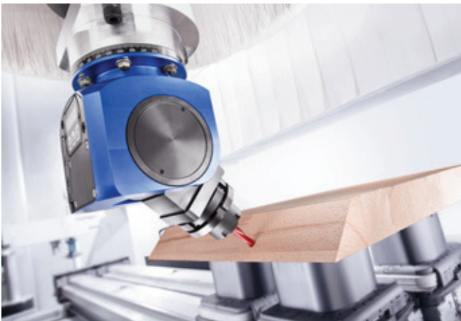
Dowel drill holes in miter
