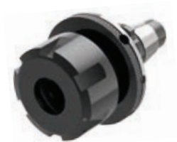
Collet chuck holder with externally located clamping nut per DIN6499 Clamping range ER 25 \varnothing 2– \varnothing 16 ER 32 \varnothing 2– \varnothing 20
