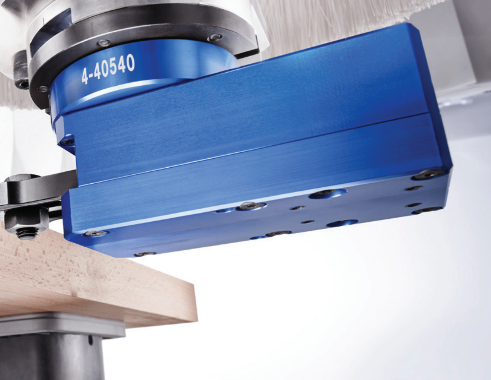
Horizontal insertion of slots for fiche hinges
