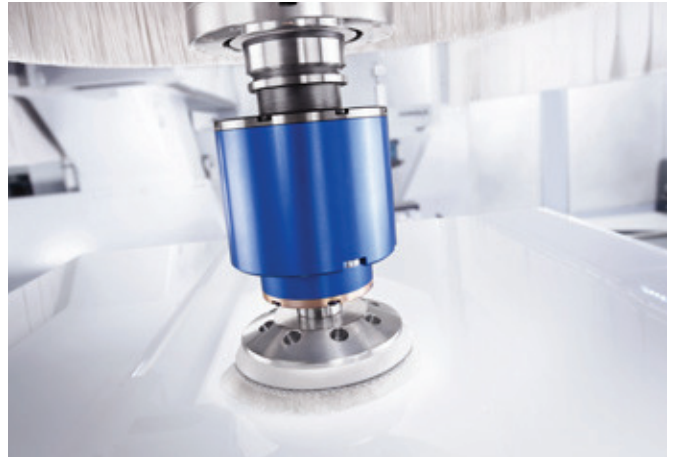
High-gloss polishing with commercially available polishing pads
