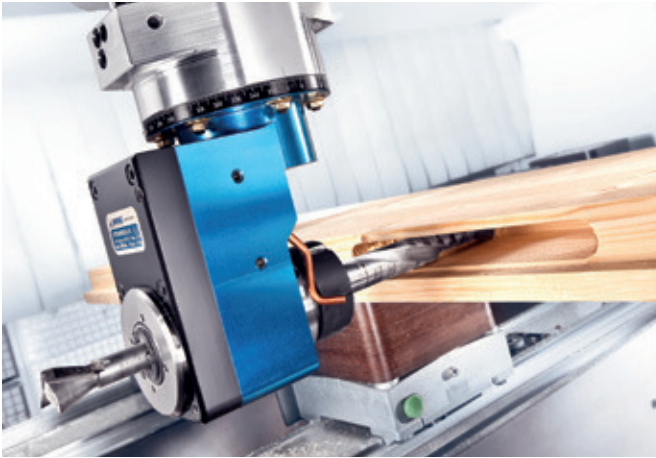
Milling lock cases and faceplates
