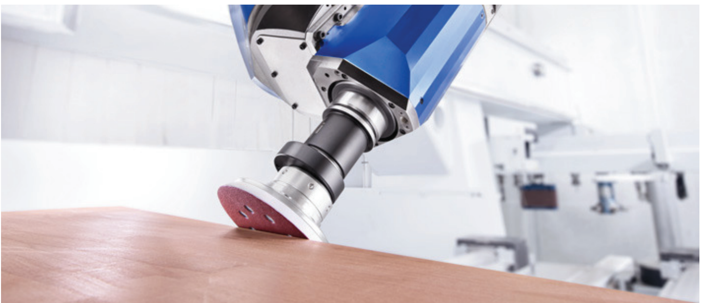
Chamfer sanding on a step
